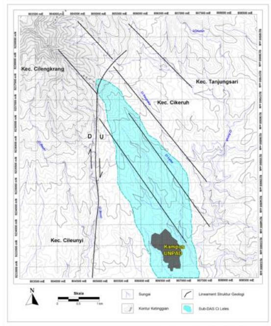
Figure 3. Lineaments in study area and possible occurrence of fault.
